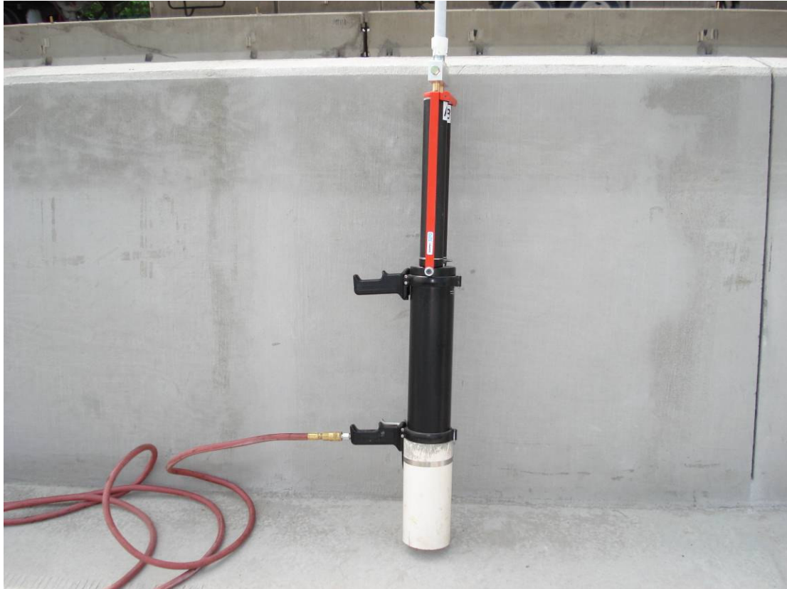
Figure 12: Gun used to install Sealant
